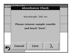
The Absorbance Check test is used to test the photometric accuracy and repeatability of the instrument.
